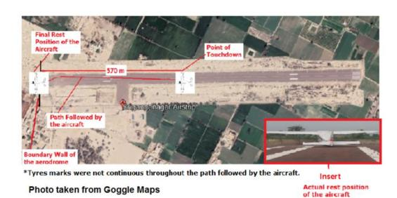
The aircraft during landing overshot the runway. As there is no RESA available, the nose portion of the aircraft hit the boundary wall of the aerodrome. The ground marks indicate that flight crew at the very last moment had tried to turn the aircraft.
